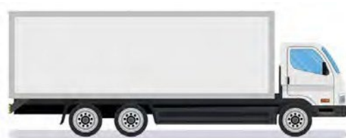
Truck with dual or tandem rear drive axle (dual or tandem drive bridge)
